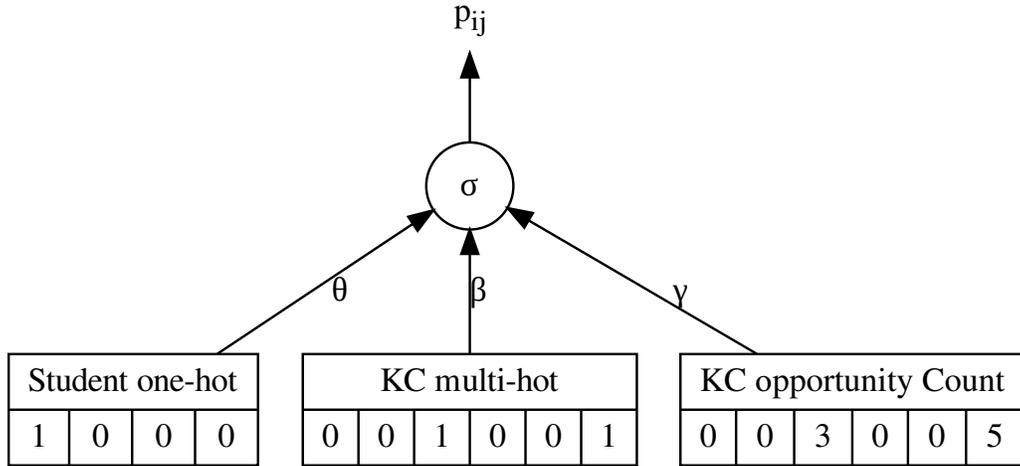
Figure 2: The AFM model posed as a feed-forward neural network with three separate input layers representing the student, the KC(s) of the item the student answered, and the student opportunity counts associated with the KC(s) of the item. The inputs are multiplied element-wise with their respective weight vectors, summed, and sent through a sigmoid activation function to predict correctness.
