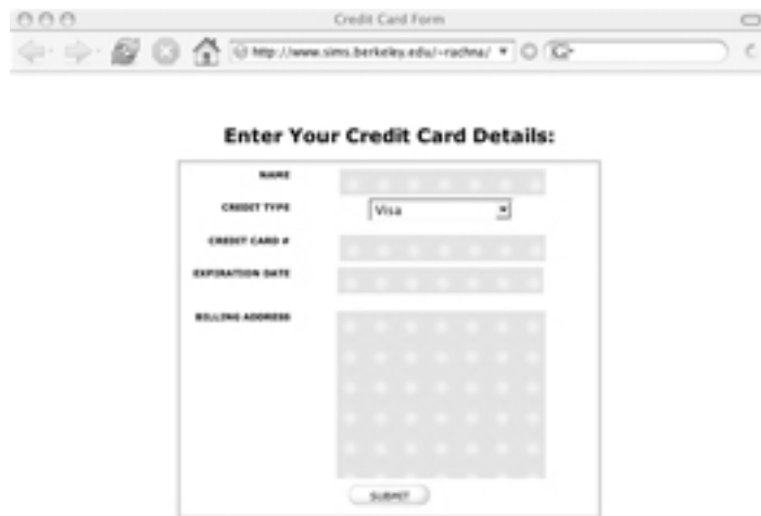
Fig. 3. The remote website displays a visual hash in the background of a form
