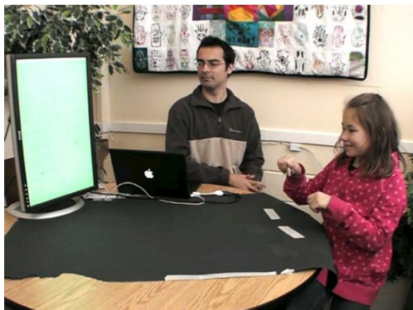
Figure 3: Infrared sensors transmit the relative locations of the student's hands to a Wii remote. The screen turns green if the hands are held at a proportional distance.
