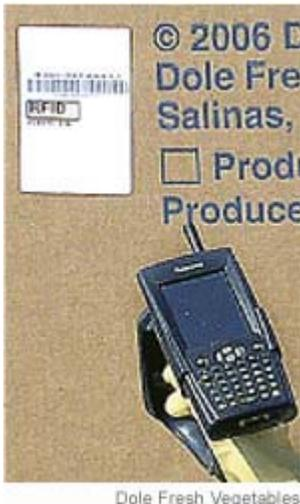
A 'scanning gun' transmits data to the company's central system.
