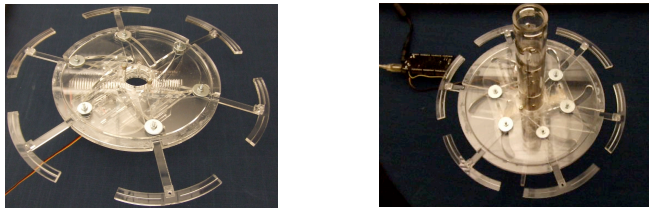
Figure 1. The left figure shows the Tangible Visualization Module (TVM) of the Weather Lamp. The right figure is the Weather Lamp with one module installed. A finished Weather Lamp will have three TVMs.
