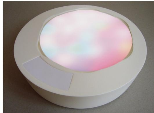
Figure 5: A model of MyInnerLife with the input surface and the touch display to enter the time.
