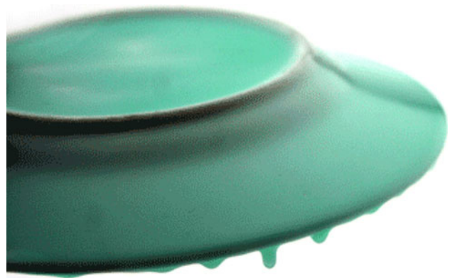
Fig. 2 The backside of the plate is coated with silicone. Once the material dries, it becomes firm but still pliable, allowing the ceramic surface to crack yet remain intact
